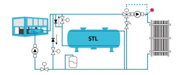
**Figure 7.** Cooling storage system scheme installed in parallel with the cooling system. (CIAT)
