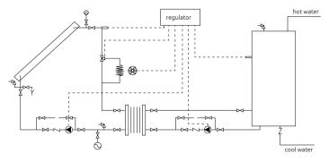
Figure 13. IMS solar thermal system scheme (CPC solar).
