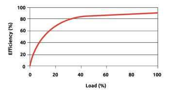
**Figure 10.** Efficiency of an electric motor according to the load (BREF, 2009).
