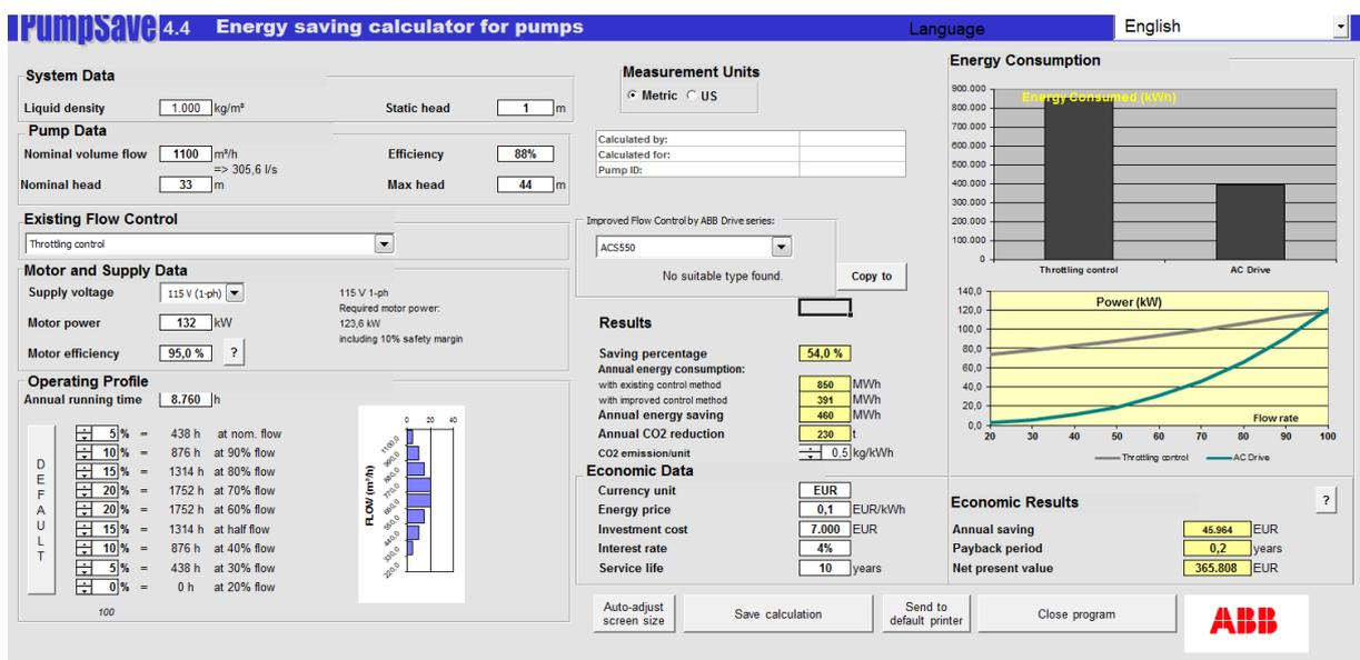
Figure 17: ABB Pump Save tool, main screen.
