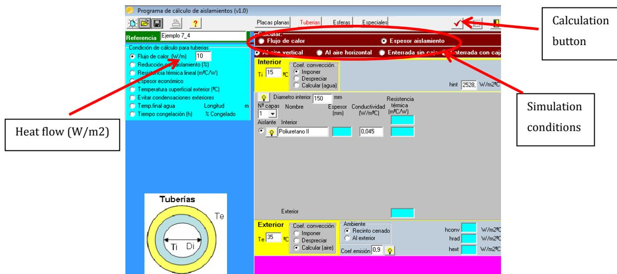
Figure 35: Aislam screen. Pipe calculation
