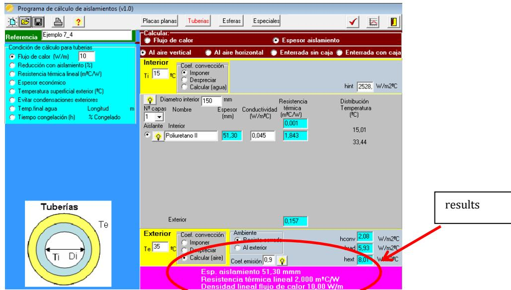
Figure 36. Aislam results screen in case: evaluate isolation thickness in piping by means of indicate what the maximum allowable thermal flow is.
