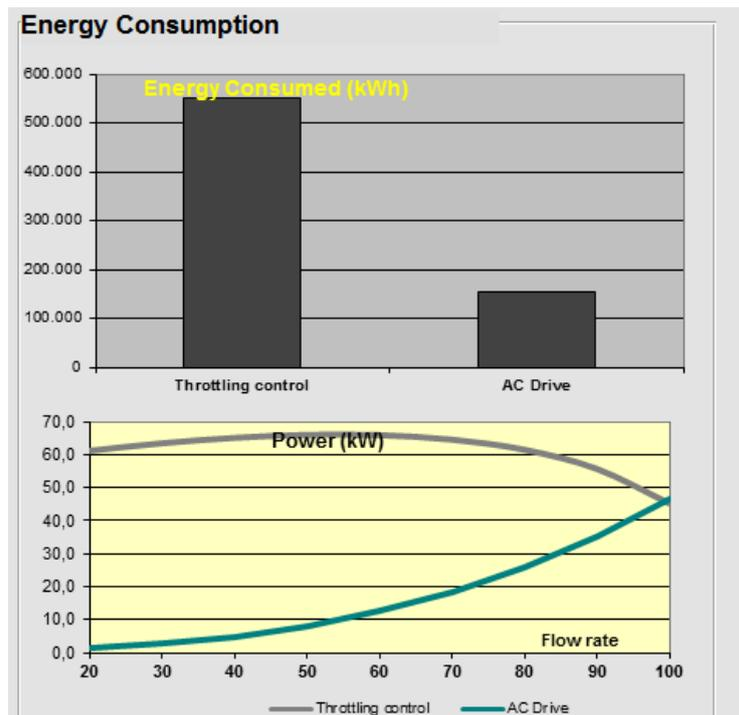
Figure 19: ABB PumpSave energy graphs
