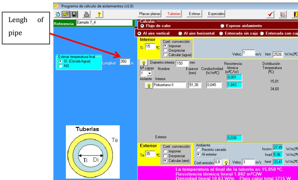
Figure 37: Aislam results screen in case: evaluate isolation thickness in piping showing final pipe temperature.
