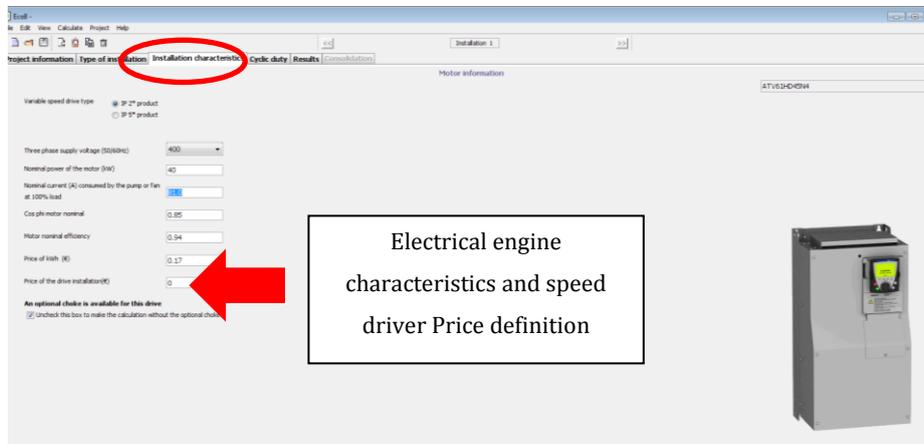
Figure 22: Eco8 installation characteristics screen
