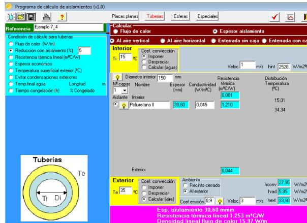
Figure 38: Aislam results screen in case: evaluate isolation thickness in piping by means of indicate what the energy consumption respect don't use isolating is.
