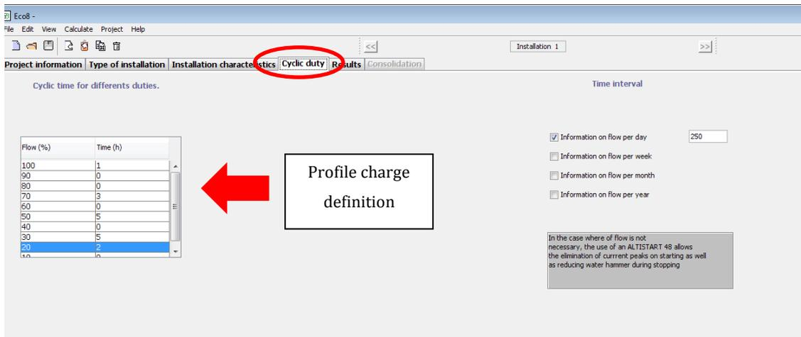
Figure 23: Eco8 profile charge definition screen
