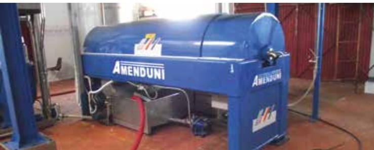
**Figura 7. Centrifugadora horizontal (Decanter)**
