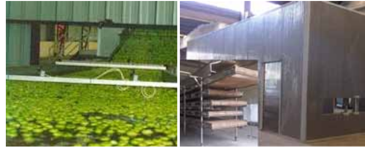
Figure 6. Water dumping of apples (on the left) and a tunnel used for drying (on the right).
